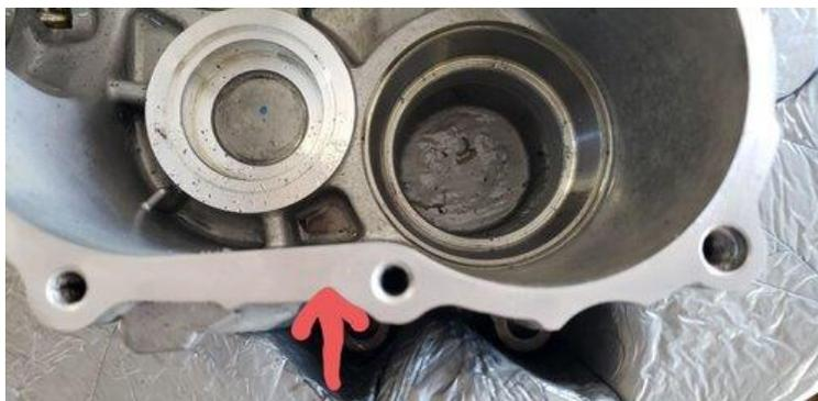
Here is a photo of an open PTU to illustrate where you want to drill the hole and why. The area is circled and is placed there to avoid the gears inside the case. It is also a very thick portion of the case:
