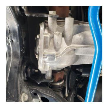
Install NPT-to-Flare fitting adapter:
